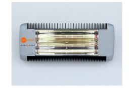
Always ensure the power cables are fixed securely (e.g. in conduit or trunking) and are safely out of reach of the horse. The cables must also be outside of the radiant heating zone of the emitter. There should be an unimpeded free air space above the Bask Zone of at least 32cm, and clearance to each side of at least 100cm. There should be a free-air space in front of the emitter of at least 100cm.
